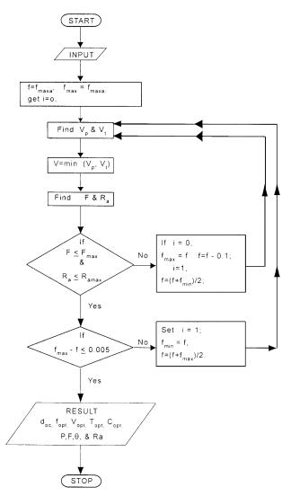
Fig. 1. Flowchart of "boundary search procedure".
