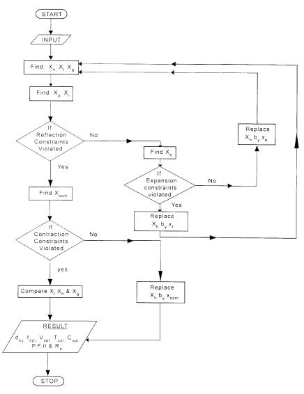
Fig. 2. Flowchart of "Nelder Mead simplex method".
