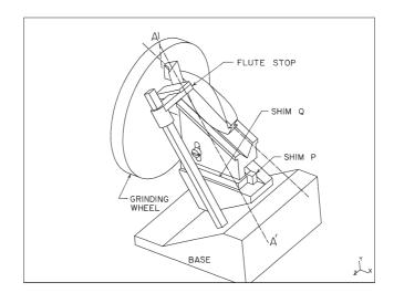
Fig. 3. Isometric view of the standard conical twist drill grinder.
