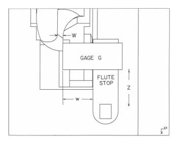
Fig. 5. Setting drill point  $\omega$  parameter.
