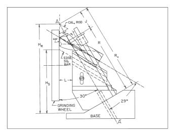
Fig. 2. Side view of the standard conical twist drill grinder.
