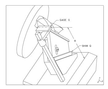
Fig. 4. Setting distance R, with drill rotated 90° about cone axis.
