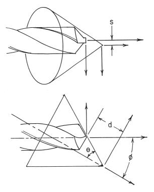
Fig. 1. Cone model of a twist drill point.
