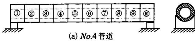
Figure 4.12 No.4, No.5, No.6, No.7 16 pipeline model
