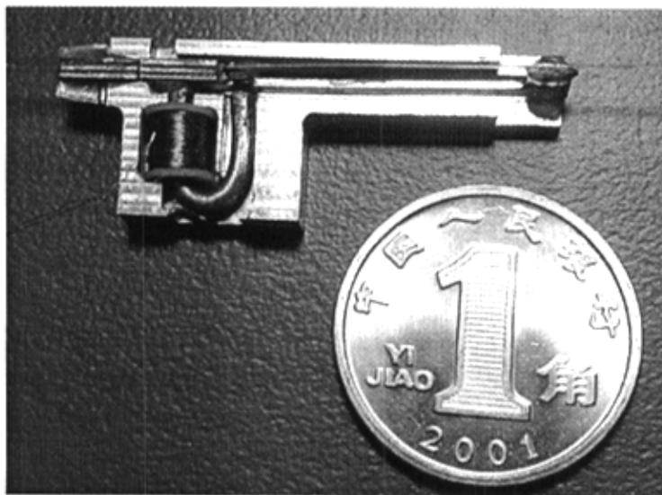
**Fig.3.7** A photo of the 1×2 fiber optic switch
