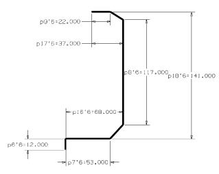
Fig. 2. Outer piece of upper rail.
