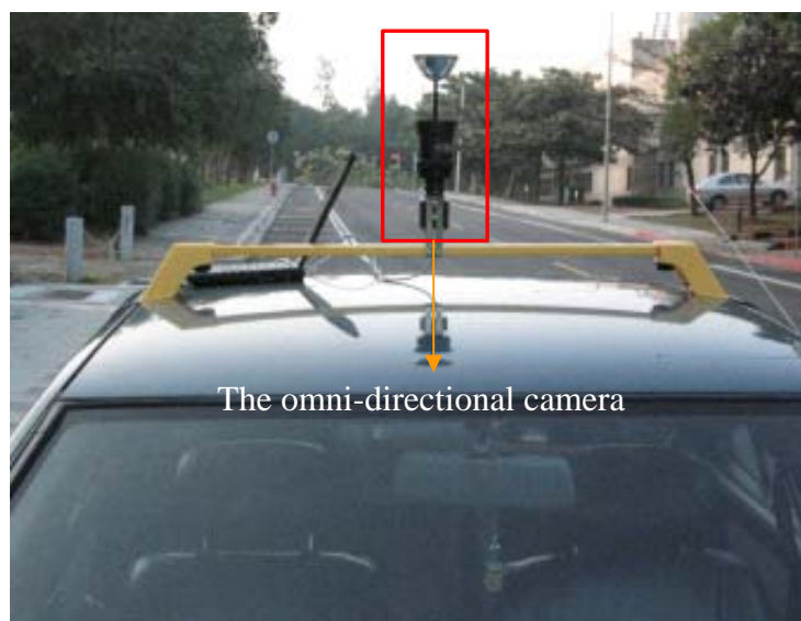
Figure 2.3 The omni-camera used in this study.
