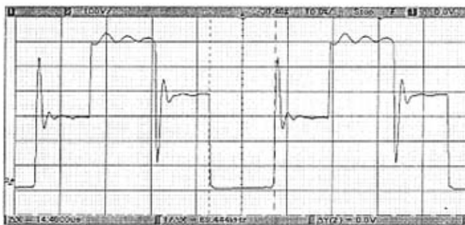
图 6-6 焊接电流 200A 时的 IGBT 管压降波形 Fig.6-5 Waveform of IGBT when welding current is 200A
