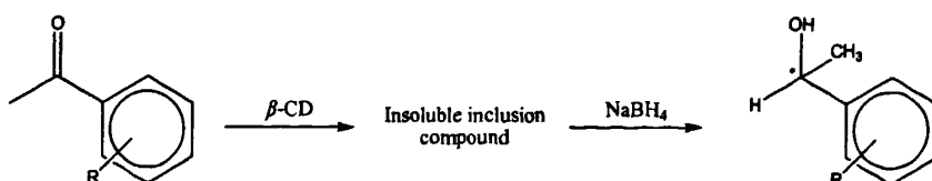
图 2-1 \beta -CD 存在下, \text{NaBH}_4 对苯乙酮衍生物的不对称还原过程 Figure 2-1 Asymmetric reduction pathway of substituted acetophenones in the presence of \beta -CD
