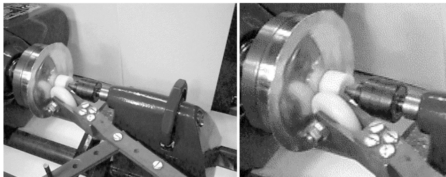
Fig. 7. The rig used for spinning 0.5 mm sheet metal.
