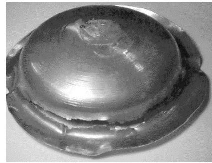
Fig. 6. Tensile failure where sheet thickness is reduced.
