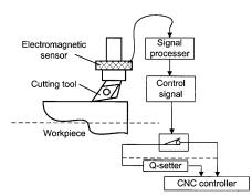
Fig. 1. Flow diagram of a fine touch sensor fixed on a CNC controller.
