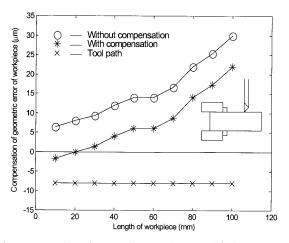
Fig. 8. Compensation of geometric error by a modified NC command.
