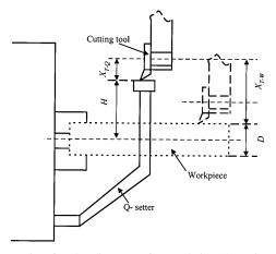
Fig. 2. Inspection for the diameter of a workpiece by using the fine touch sensor with the Q-setter of a machine tool.
