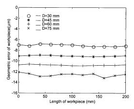
Fig. 5. Geometric errors of the workpiece along the z-axis.
