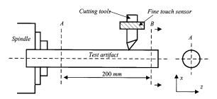
Fig. 4. Diagram of the geometric error measurement of the workpiece using FTS\_Q.
