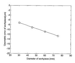
Fig. 6. The average geometric error for the different diameters.
