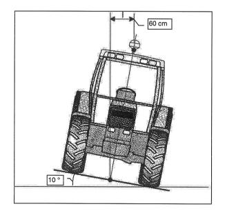
Fig. 1. Difference in position for two locations due to sloping terrain.
