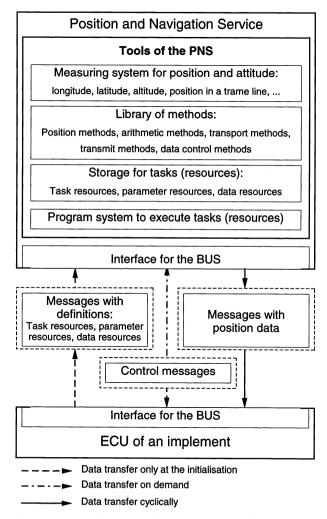
Fig. 3. Streture of a PNS and its data exchange with one ECU.
