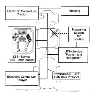
Fig. 2. Scheme of an agricultural network in a tractor-sprayer combination.
